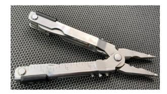
The main features of this Multi-Tool is that it has all the tools that I use on a daily basis and it collapses down to the small, compact form that fits on my belt. It is made of stainless steel and doesn't rust but is still magnetic enough so it will work with other magnetic tools. It contains 18 different tools as well as the ability to add bits to the Phillips head screw driver and blades to the saw blade holder.
